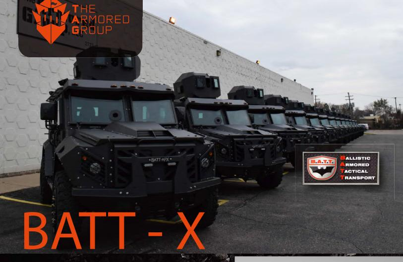
The BATT®-X is a multi-purpose APC with incorporated v-hull base. For 2020, additional length has been added to the to allow the BATT®-X to carry 10-14 Officers (depending on size of operators and amount of gear). It is designed for law enforcement agencies and tactical teams to carry out missions in both rural and urban settings.
